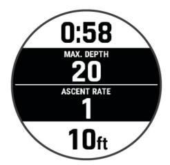
**In-dive screen**: Displays the information about the current dive, including the elapsed time, current and maximum depth, and rate ascent or descent. You can edit the data screen layout and data fields (*Customizing the Data Screens*, page 105).
