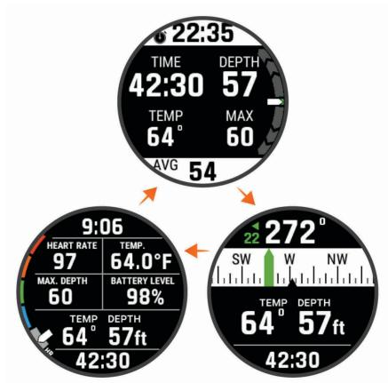
**Dive stopwatch**: Displays the bottom time stopwatch; current, maximum, and average depth; and rate of ascent or decent (*Using the Gauge Dive Stopwatch*, page 18).
