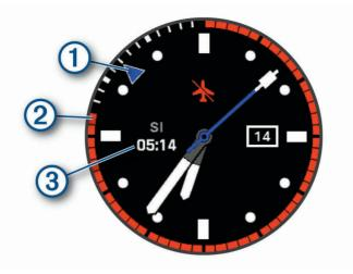
D Alternate time zone pointer. References the 24-hour time markings on the watch (*Adding Alternate Time Zones*, page 91).
